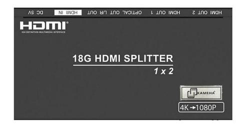
The 18Gbps HDMI 1×2 Splitter can distribute 1 HDMI source signal to 2 HDMI display devices. It supports resolution up to 4K2K@50/60Hz (4:4:4). This product supports audio extract from HDMI source to optical and analog output. Two EDID modes (COPY/AUTO) can be selected. All output ports support signal bypass and video downscale (4K->1080P) function.
